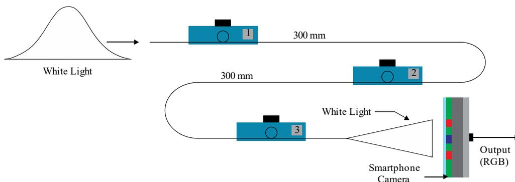
Fig. 1. Diagram of the experimental set-up used for multiplexing the intensity-modulated sensors.
