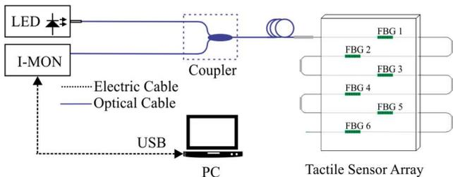
Fig. 4. Interrogation unit connected to the sensor array.
