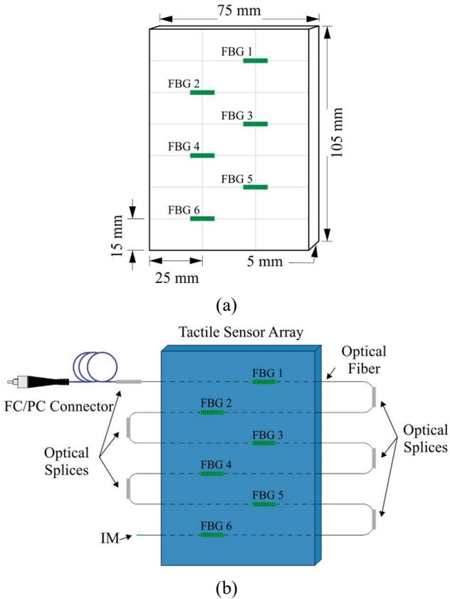
Fig. 3. Diagram showing: (a) the vertical and horizontal distance between the FBGs in the sensor array; (b) the fiber connections of the sensor array.
