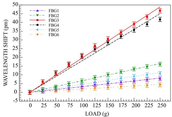
Fig. 6. FBGs responses and calibration curves for different loads applied at the central position of the tactile sensor array.
