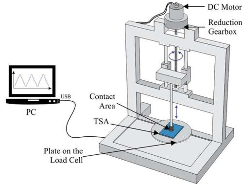
Fig. 5. Schematic of z-stage system.
