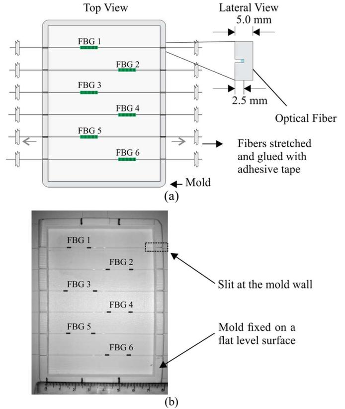
Fig. 2. (a) Diagram showing the FBGs placed at the 3D printed mold and a detail of the slit at the mold wall; (b) Picture of the mold with the installed FBGs.
