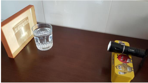
Fig. 1. Setup for the measurement of the focal length of a positive lens.
