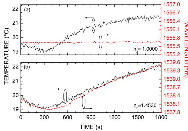
Fig. 1 – Temporal evolutions of temperature and wavelength for (a)  $n_s = 1.0000$  and (b)  $n_s = 1.4530$ .
