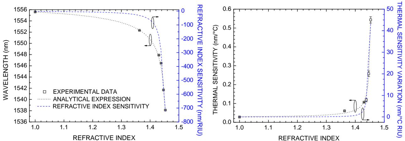
Fig. 2 – (a) LPFG responses with surrounding RI, (dotted curve) fitting result obtained from equation (2), and (dashed curve) LPFG refractive index sensitivity. (b) Thermal sensitivities obtained for air, ethanol and hydrocarbons samples and (dashed curve) temperature influence with RI. Dashed and dotted curves are just a visual guide.
