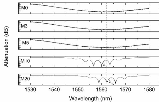
Figure 2. Transmission spectra of CLPG immersed in MX samples at 20 °C.
