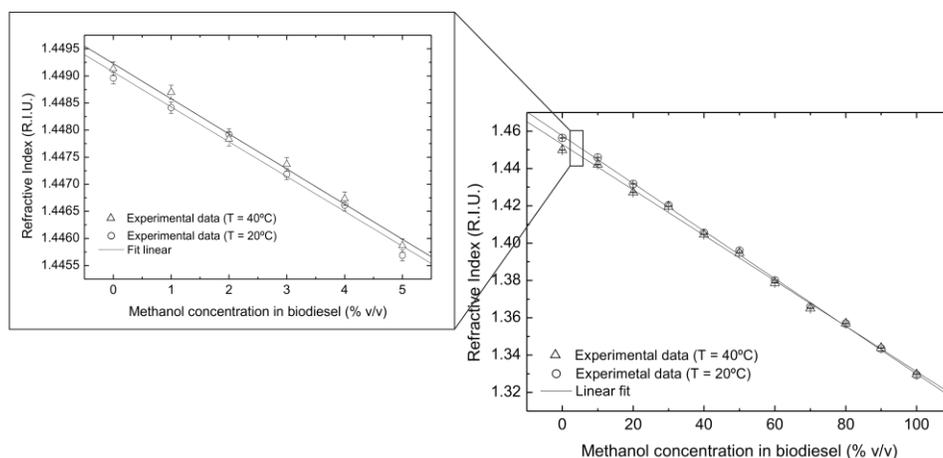
Figure 1. Refractive indices of biodiesel-methanol samples measured with the Abbe refractometer at 20.0 °C and 40.0 °C.
