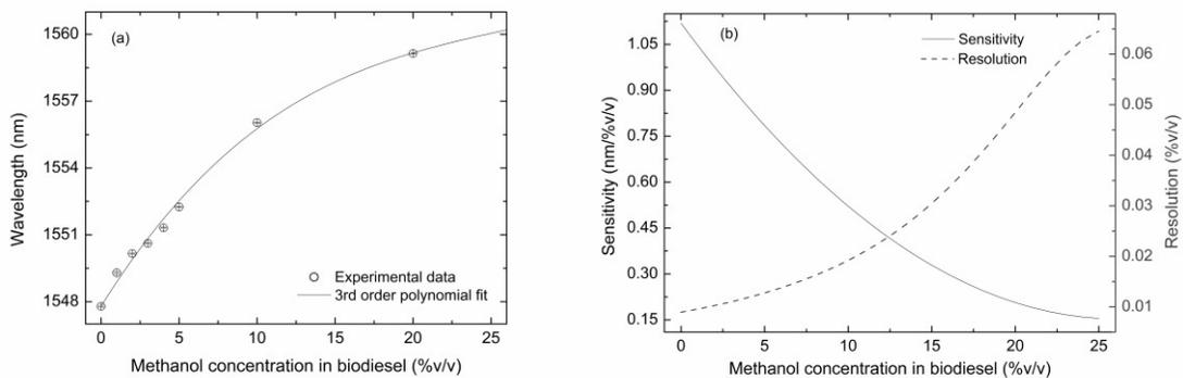
Figure 3. (a) Response curve of CLPG immersed in MX samples at 40.0 °C, (b) Sensitivity (solid line) and resolution curves (dashed line).
