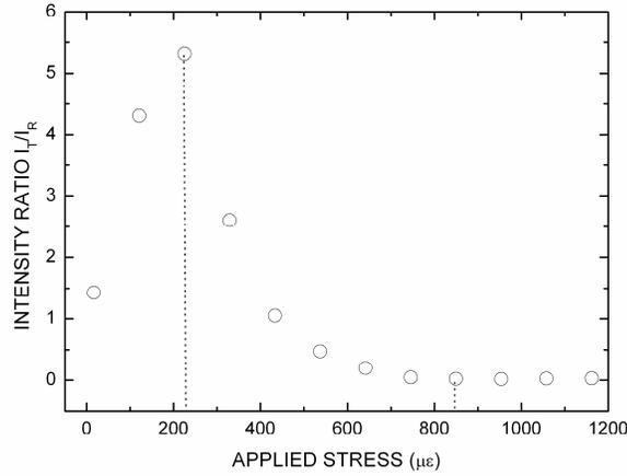
Fig. 6. Ratio of the intensities between the transmitted and reflected beams for several screw angle positions in the sensing head, obtained with the experimental setup of Fig. 2 and grating 1 (bandwidth of 0.11 nm and Bragg wavelength of 1548.9 nm at 21 °C).
