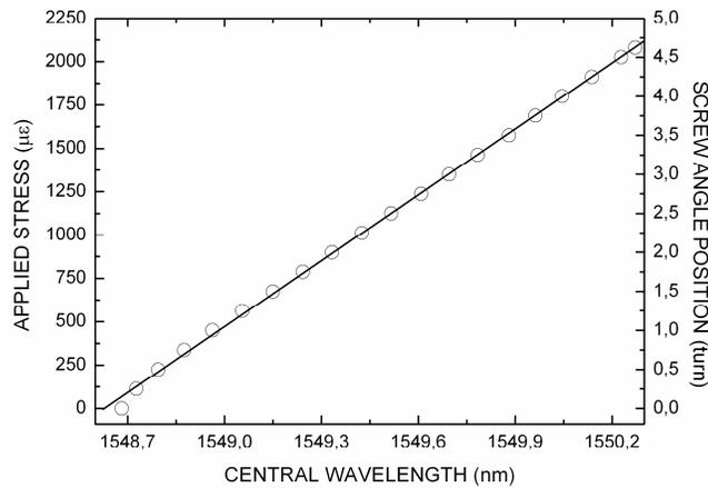
Fig. 3. Wavelength response of the sensing FBG (grating 1, bandwidth of 0.11 nm and Bragg wavelength of 1548.9 nm at 21°C) mounted in the sensor head.
