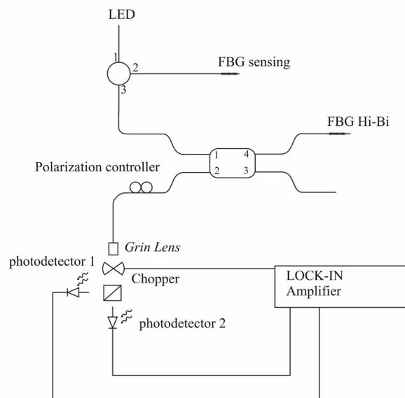
Fig. 2. Diagram of the interrogation system intensity coded experimental setup.
